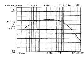
In this example, we're using the analyzer's internal A-weight filter. The choice of a linear or logarithmic X-axis is not critical—math operations are not affected by this decision.
