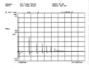
This trace shows the time domain result of a multiple impact, such as when the hammer bounces during impact.
