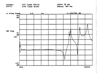
This trace shows the frequency response of a single, good hammer tap.
