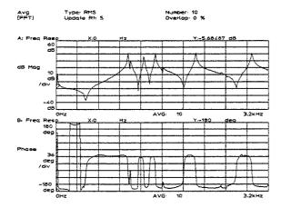
This turns on autoscaling for both traces. The analyzer scales the data to best fit the display.
