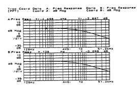
This displays the measurement data on a logarithmic scale. This is more useful for viewing the frequency response of some devices, particularly audio-frequency devices.
