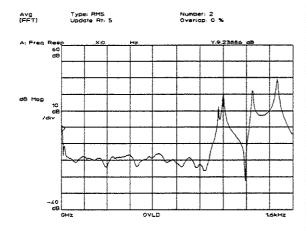
This trace shows the frequency response with channel 1 overloaded. Notice that the overload causes distortion in the frequency response.
