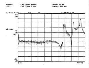
This trace shows the frequency response of multiple impact, such as when the hammer bounces during impact. Notice that a multiple impact produces a ripple on the frequency response.
