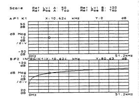
This shows the integrated function. The curve appears to be exponential because the analyzer's default trace coordinate is dB magnitude. This is because in dB magnitude, the Y-axis is logarithmic.
