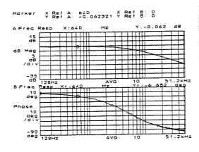
In a moment, we're going to change the lower trace from dB magnitude trace coordinate to the phase coordinates.
