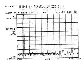
Note how the Y-axis marker readout indicates a relative reading of approximately -72 dB, and the X-axis marker readouts are now set to zero—this point now becomes the reference.
