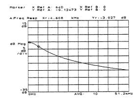
This moves the marker to the largest part of the frequency response trace. Because we are looking at a frequency response trace, the X-marker indicates amplitude in relative terms (dB).
