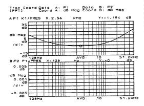
Note how the product of the inverse trace and the orignal frequency response trace is a flat line.
